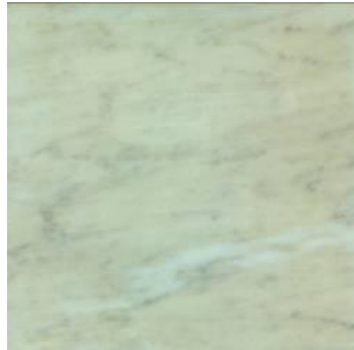
Figure 18: a Carrara Bianco C tile after the alkaline water test
