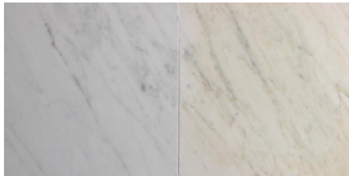
Figure 14: an Bianco Carrara C tile before the alkaline water test (left) and a tile after the test (right) (not the same tiles).
