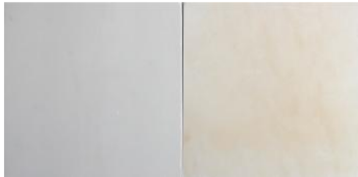
Figure 16: a Bianco P tile before the alkaline water test (left) and a tile after the test (right) (not the same tiles).
